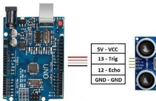
**Figure 2.** Connection diagram
