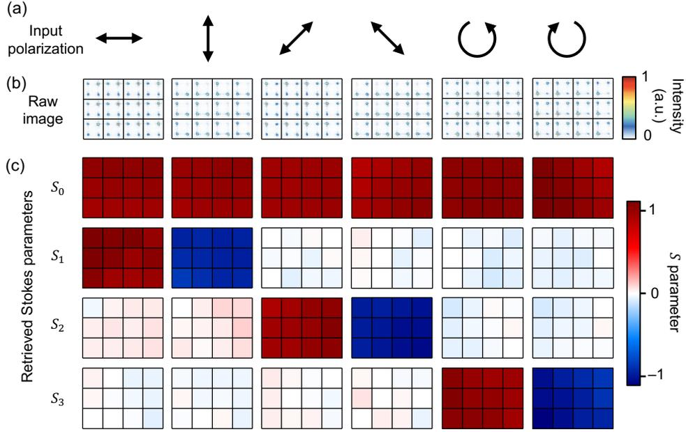
Fig. 6. Measured results of  $3 \times 4$  superpixel array. (a) Input SOP. (b) Measured intensity distributions at the focal plane. (c) Retrieved Stokes parameters for each input SOP.
