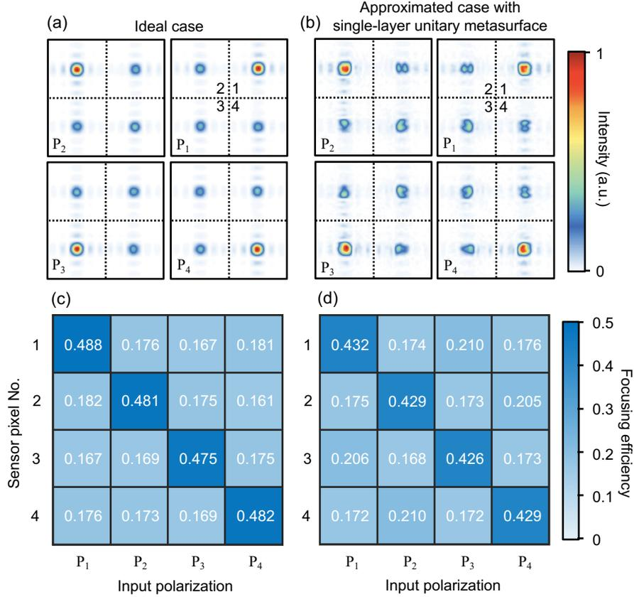
Fig. 3. Simulated results of designed metasurfaces. (a, b) Intensity distributions at the focal plane for the four different input SOPs,  $P_n$  ( $n = 1, 2, 3, 4$ ). (c, d) Focusing efficiencies to all pixels for each input SOP. (a) and (c) assume the ideal case with  $\tilde{\mathbf{J}}_d(x, y)$ , whereas (b) and (d) assume the approximated case using a single-layer metasurface with  $\tilde{\mathbf{J}}_{MS}(x, y)$ .
