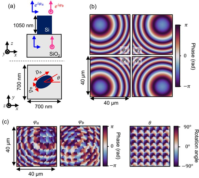
Fig. 2. Schematic and design of meta-atoms. (a) Si elliptical nanopost on a quartz substrate used as a meta-atom. (b) Required phase profiles  $\varphi_n(x, y)$  for polarization states  $P_n$  ( $n = 1, 2, 3, 4$ ). (c) Spatial distributions of the required phase shifts ( $\varphi_a(x, y)$ ,  $\varphi_b(x, y)$ ) and the orientation angle  $\theta$  of meta-atoms.
