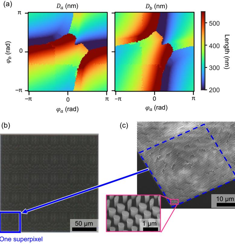
Fig. 4. Fabricated metasurface. (a) Lookup table used to determine the geometry of each meta-atom, showing required  $(D_a, D_b)$  to obtain given phase shifts  $(\varphi_a, \varphi_b)$ . (b) Optical microscope image and (c) scanning electron microscope (SEM) images of the fabricated metasurface.
