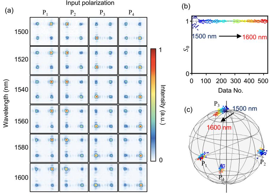
Fig. 7. Measured wavelength dependence. (a) Intensity distributions at a wavelength from 1500 nm to 1600 nm for the four different input SOPs  $P_n$  ( $n = 1, 2, 3, 4$ ). (b,c) Retrieved  $S_0$  parameter and the Stokes vectors  $(S_1, S_2, S_3)^t$  on the Poincaré sphere measured by all 12 superpixels at wavelength from 1500 nm to 1600 nm.
