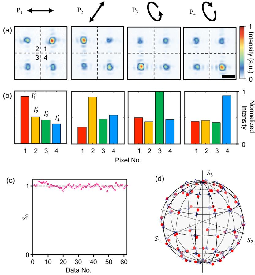
Fig. 5. Measured results of one superpixel. (a) Intensity distributions at the focal plane for the four different input SOPs,  $P_n$  ( $n = 1, 2, 3, 4$ ). (b) Integrated intensities at four pixels for each input SOP. (c,d) Retrieved  $S_0$  and Stokes vector  $(S_1, S_2, S_3)^T$  on the Poincaré sphere. Red: retrieved. Blue: actual.
